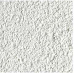
Example of: Thin Coat Render (Photograph indicative) Actual colour to be confirmed. All render finishes to be terminated in pressed metal flashing's and corner trims where needed
