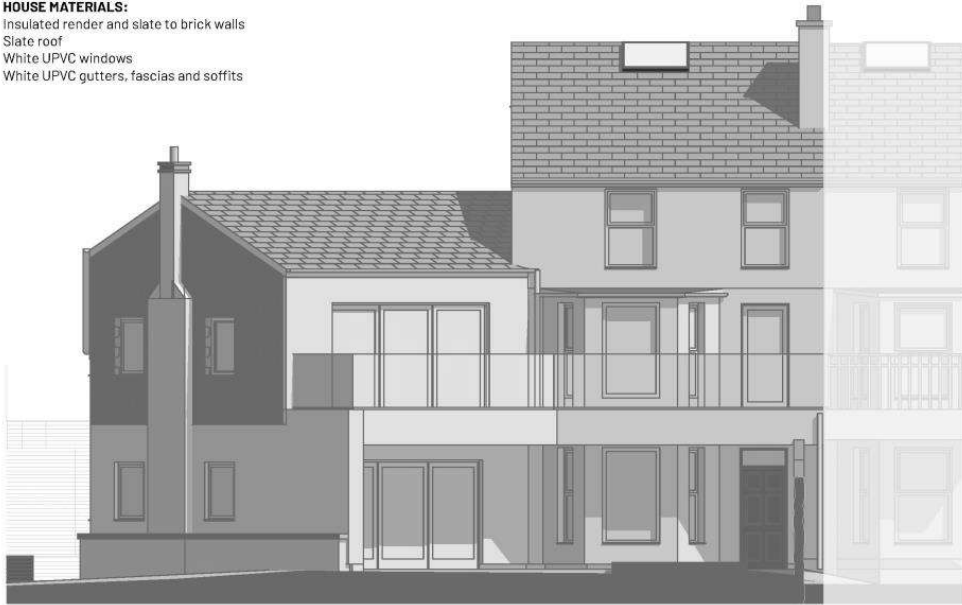
NW House Elevation 1:100
