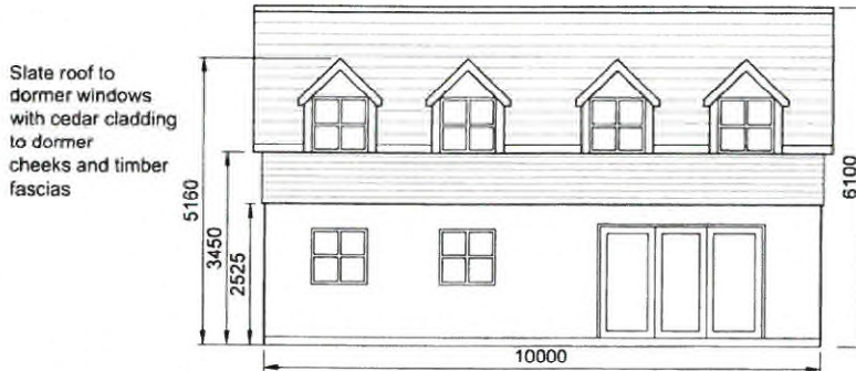
3. Rear Elevation - North West
