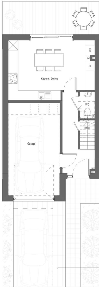
GROUND FLOOR PLAN - 1:50 27.8m 2 (+17.5m 2 garage)
