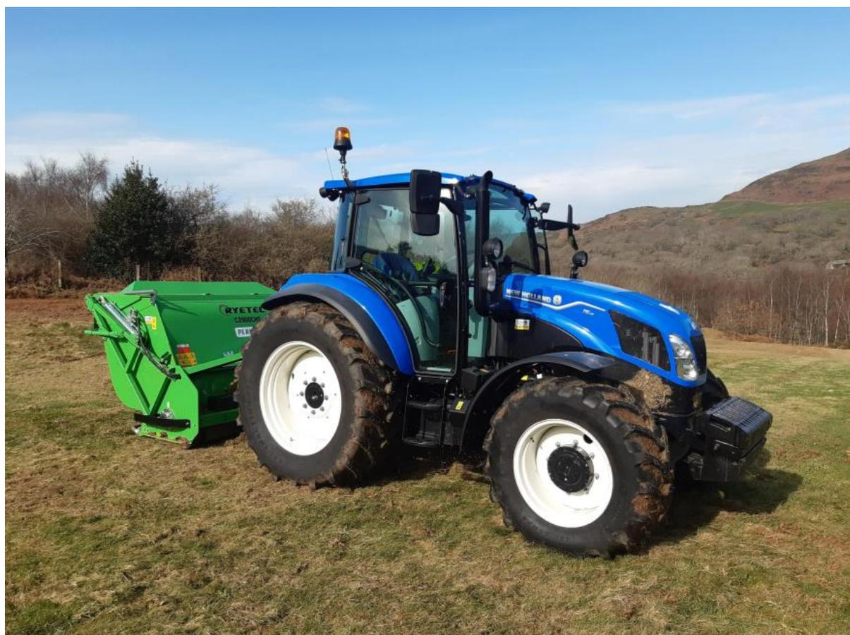
**New Holland Tractor with Rytec cut-and-collect attachment**
